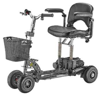
The SPRINT is smaller than the Scooter SPORT. Equipped with four 200 mm wheels, it is the perfect fit for driving outdoors. Due to the compact and comfortable design and a suspended seat, as well as the ability to be dismantled in 3 parts (none of which weigh more than 10 kg), the SPRINT is the ideal compagnion for daily use and travel.
